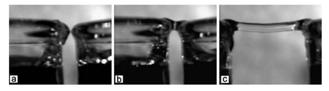
**Figure 6.** Formation of a water bridge between two Teflon beakers. (a) No current applied, (b) rise of the water surface mainly in the anodic beaker at approximately 15 kV dc, (c) spark, (d) water jet ejection leading to (e) a stable connection between the beakers (left cathode, right anode beaker) (from [89]).
